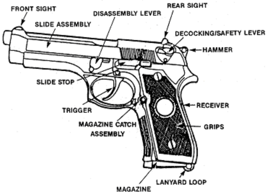
Figure 4-1.--M9 Service Pistol.
